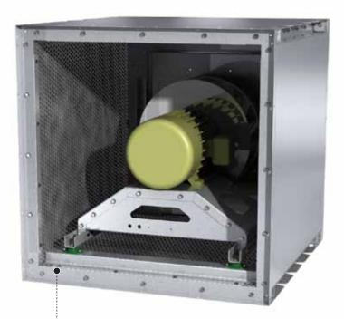
FAN-CY THIS The new Housed Plenum Array model HPA is designed for fan installations in air handler applications. Model HPA features a direct-drive galvanized plenum fan mounted inside a sound-attenuating housing. Integrated isolators between the fan and housing reduce vibration.
