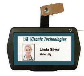
**REDUCING RISK** With its distinctive photo-ID form factor, the Elpas Quad-Tech personal badge is a hybrid active-passive tag that enables fast real-time locating system and access control interoperability. The badge provides staff location down to the subroom level with duress call signaling for workers at risk of attack or injury.
